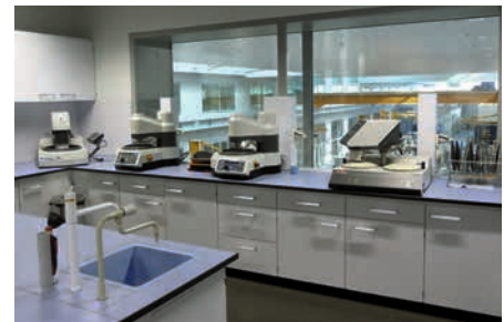
Fig. 23: Metallographic laboratory equipment (grinding and polishing).
